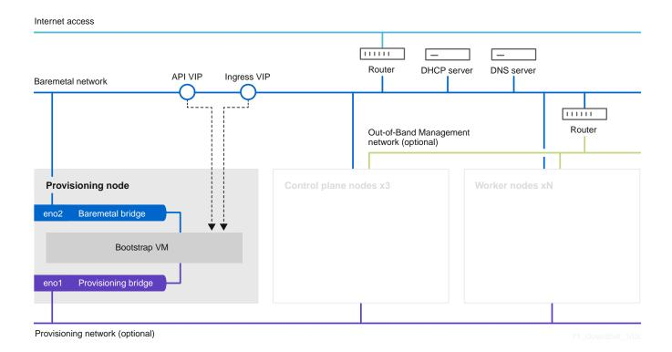
When the installation of OpenShift control plane nodes is complete and fully operational, the installer destroys the bootstrap VM automatically and moves the virtual IP addresses (VIPs) to the appropriate nodes. The API VIP moves to the control plane nodes and the Ingress VIP moves to the worker nodes.
