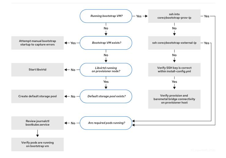
*Workflow 2 of 4* illustrates a troubleshooting workflow for bootstrap VM issues, bootstrap VMs that cannot boot up the cluster nodes, and inspecting logs.
