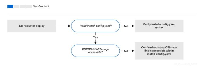
*Workflow 1 of 4* illustrates a troubleshooting workflow when the install-config.yaml file has errors or the Red Hat Enterprise Linux CoreOS (RHCOS) images are inaccessible. Troubleshooting suggestions can be found at
