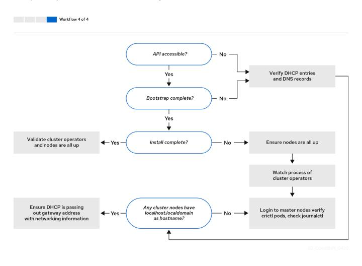
*Workflow 4 of 4* illustrates a troubleshooting workflow from a non-accessible API to a validated installation.
